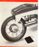
The rear wheel is easily withdrawn when the quickly detachable rear number plate has been removed.
