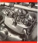
Simple and positive valve adjustment is provided by eccentric rocker spindles in the polished alloy head.
