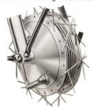
This unusual patented crankshaft is unique because it tapers in hollow section, from large to small, in perfect stress harmony.
