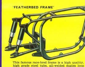
This famous race-bred frame is a high quality, high grade steel tube, all-welded duplex loop construction, liberally gusseted at the rear for optimum rigidity of the swinging arm. Note the unique head construction giving rigidity in all planes, one of the main reasons for the wonderful steering characteristics of Norton. The rear fork ends are solid forged for maximum strength.
