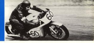
Engine. 249 c.c. twin cylinder, o.h.v. engine with integral gearbox; twin high-level camshafts; 60 mm. bore; 44 mm. stroke and a compression ratio of 8.75 to 1. Maximum b.h.p. is developed at 7,000 r.p.m. with a maximum speed of approximately 75 to 80 m.p.h. and a petrol consumption in the region of 70 to 90 m.p.g. New type contact breaker allows for individual timing of each cylinder. Coil ignition system incorporating an emergency starting device.
