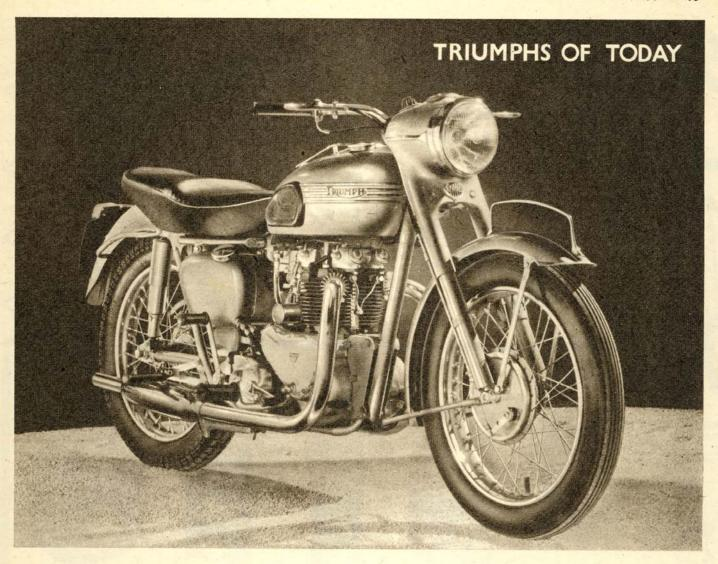
O.H.V. vertical twin engine 71 x 82 mm.—650 c.c. 34 B.H.P.—6,300 R.P.M.
