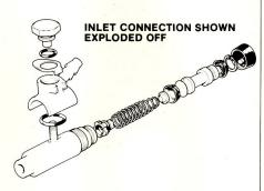
Remove the rubber boot and the circlip
