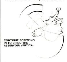
Make a further slight turn inwards to align the hole for the set screw with the centre of the flat, or slot, denoted by the pencil line. Fit the screw (ideally apply Loctite CV) and torque up 2.26 Nm. -20 lb.ins., making sure that on cylinders with a slot machined in the body that the screw locates properly into the slot.
