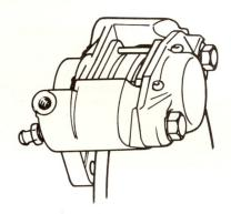
A wiper seal and a metal retainer are fitted at the mouth of each caliper bore to prevent the ingress of dirt, etc.
