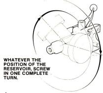
4. Continue screwing in the cylinder the part of a turn necessary to bring the reservoir vertical so as to line up with the tapped boss.
