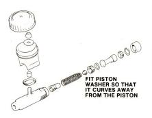
Remove the rubber boot and the circlip from the bore mouth, then withdraw all the internal parts, carefully noting their positions. Remove the secondary seal from the piston taking care not to damage the seal groove.
