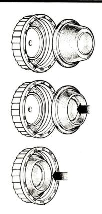
Replace the cap on the reservoir. Operate the brake lever several times to adjust the friction pad positions in the caliper if applicable, and to test for correct operation of the master cylinder.
