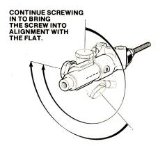
5. Fit the screw, ideally apply Loctite CV and torque up to 2.26 Nm (20 lbf ins), making sure that if applicable the screw locates correctly into the slot.
