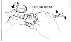
With all lost movement eliminated, note the position of the reservoir in relation to the tapped boss on the bracket.
