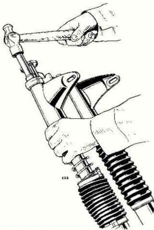
Fig. G3. Dismantling the telescopic fork using service tool Z19.
