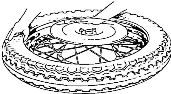
Fig. F22. Placing the security bolt in position.
