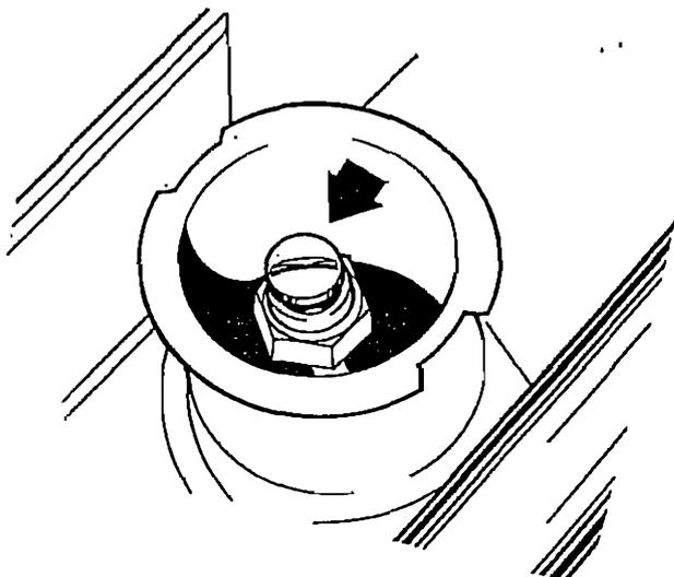
Fig A12. Rear chain oil feed adjustment
