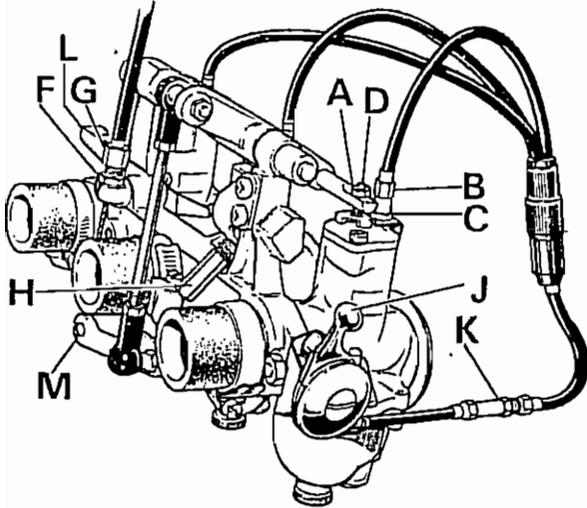
Fig. B10. Inlet manifold assembly
