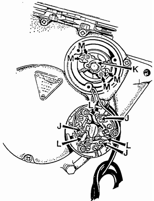
Fig. A9. Contact breaker lubrication points
