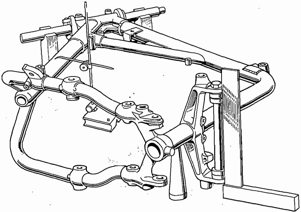
Fig. E14. Checking the front frame alignment
