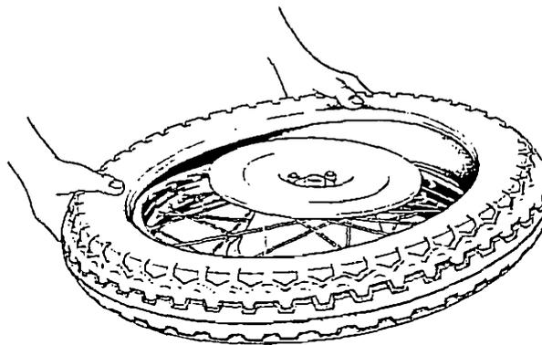
Fig. F17. Final removal of the tire
