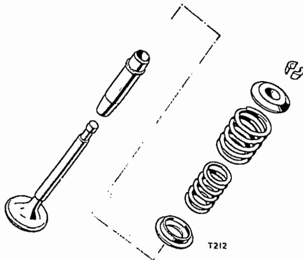
Fig. B15. Valve components
