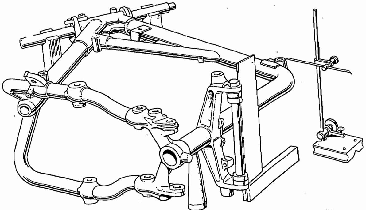
Fig. E15. Checking the front frame alignment
