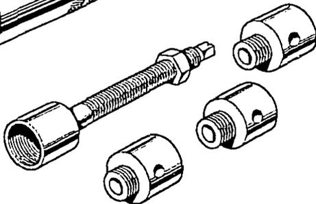
60-D2213 (61-3801) Camshaft pinion extractor and replacer with adaptors
