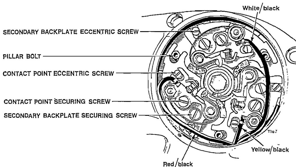
Fig. H4. Contact breaker assembly type 7CA
