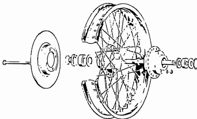
Fig. F9. Exploded view of front wheel bearing arrangement
