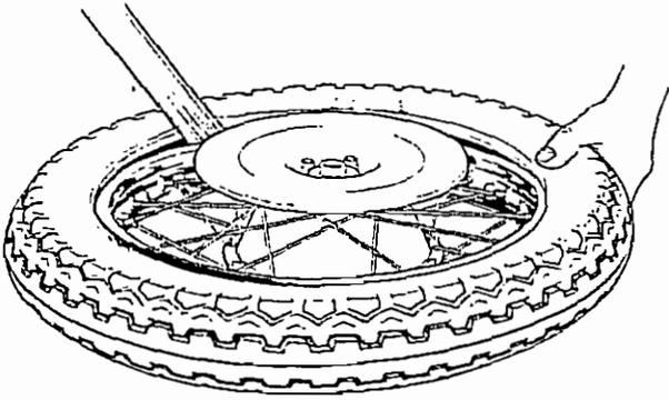
Fig. F21. Refitting the second bead over the wheel rim.
