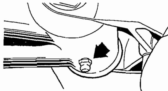
Fig. A13. Swinging fork pivot lubrication nipple
