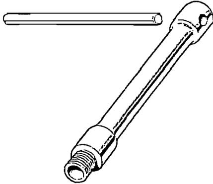
60-D1833. Valve seat cutter (inlet) (61-7026)
