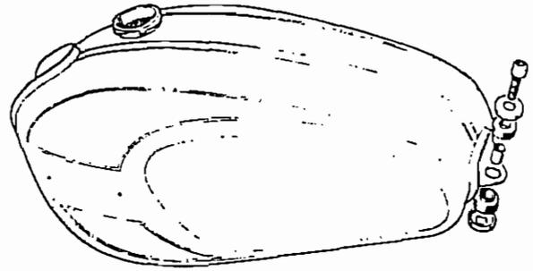
Fig. E2. Assembly order of fuel tank mountings
