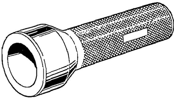
61-6020 Timing side main bearing outer spool drift
