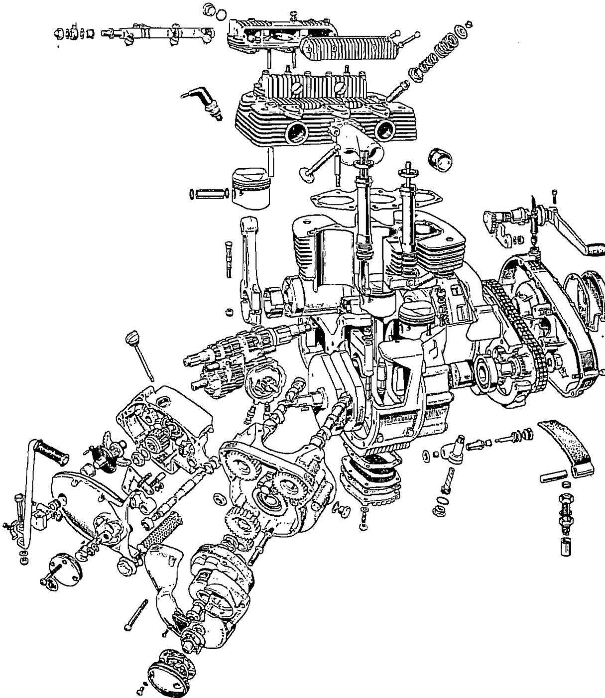
Fig. B1. Exploded view of the Trident engine-transmission unit
