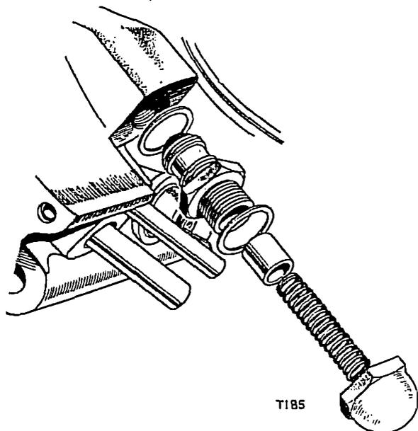
Fig. A5. The oil pressure relief valve
