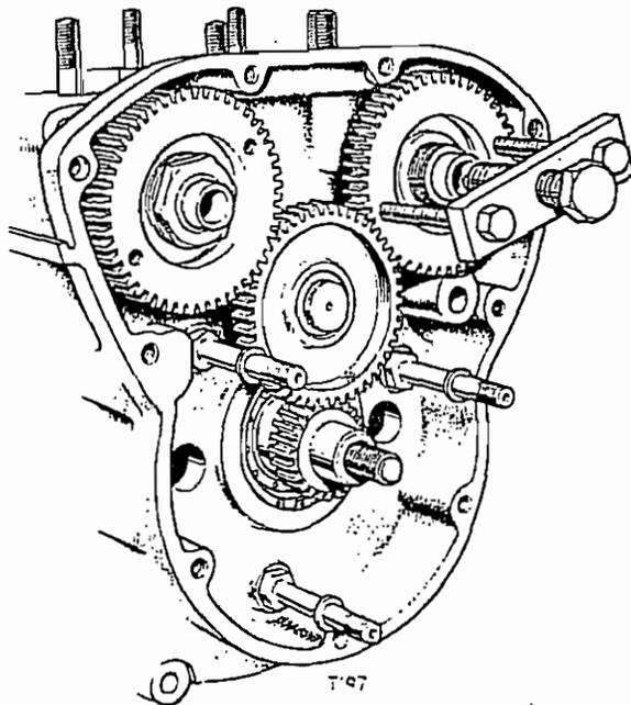
Fig. B31. Extracting camshaft pinion using tool 61-3808
