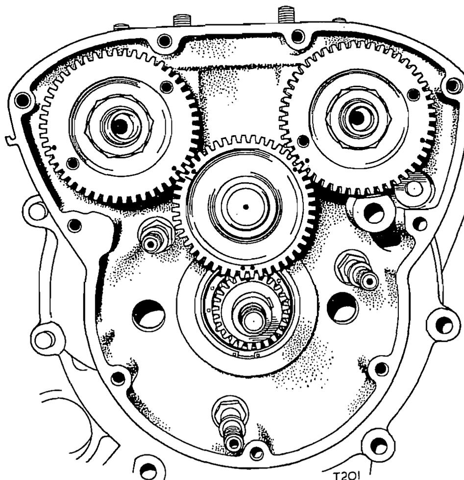
Fig. B33. Valve timing marks
