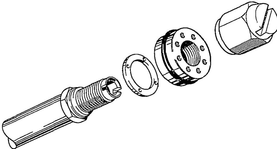
Fig. G3. Assembly of bleed valve
