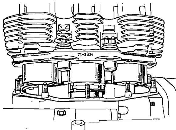
Fig. B20. Refitting cylinder block
