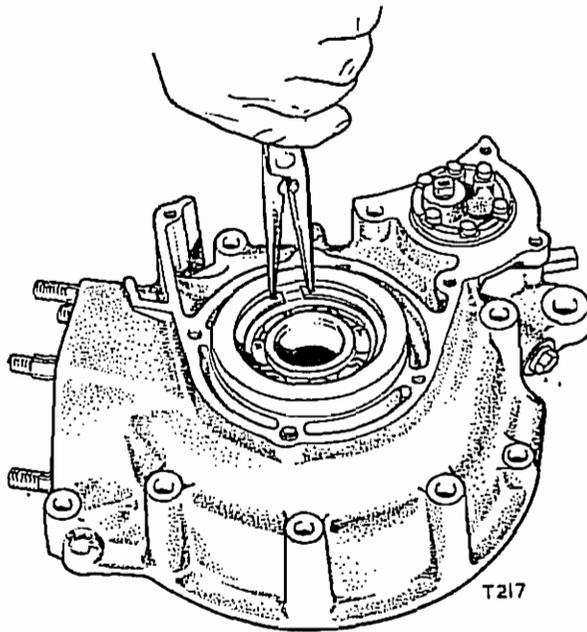
Fig. B40. Removing a circlip
