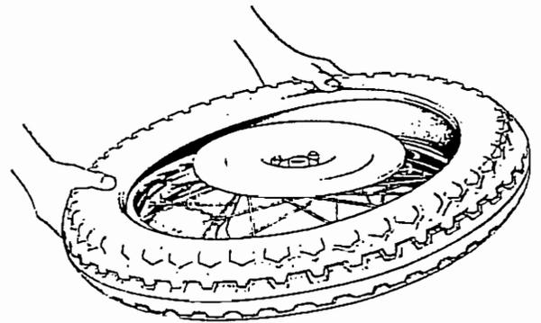
Fig. F19. Refitting the tire to the wheel.
