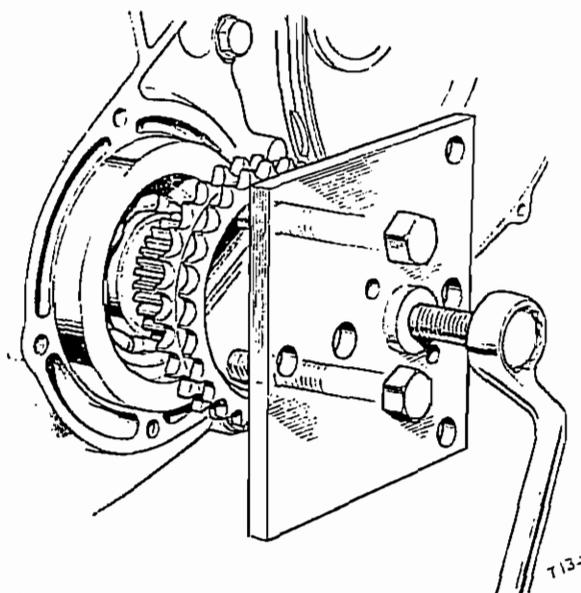
Fig. C7. Extracting the engine sprocket
