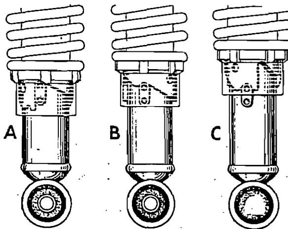
Fig. E6. Adjusting the rear suspension units
