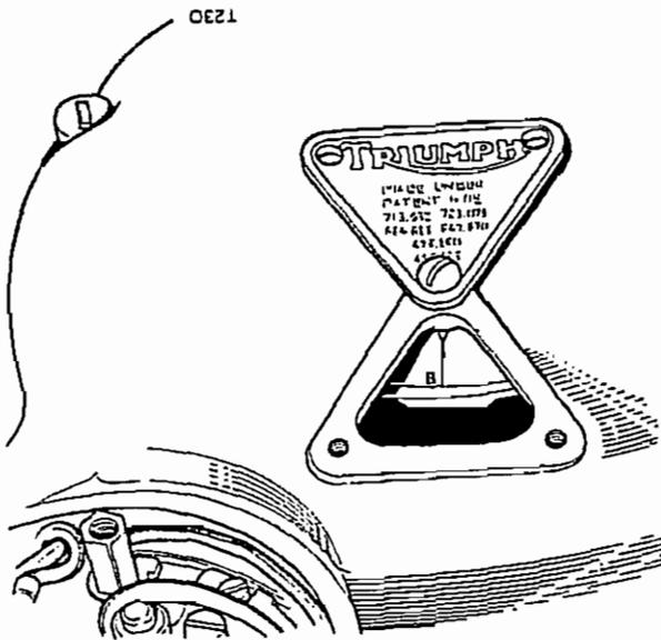
Fig. B27. Timing mark on the rotor
