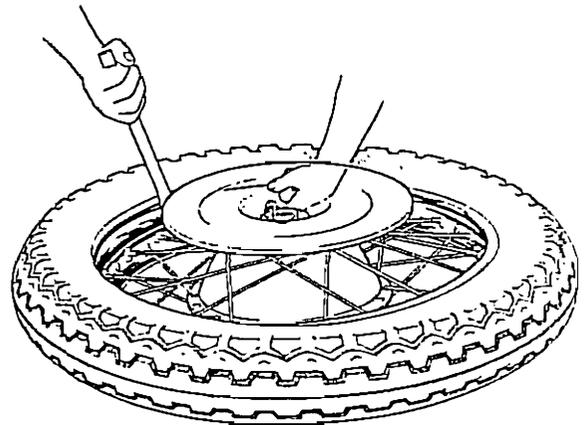
Fig. F23. Refitting the second bead with the security bolt in position.
