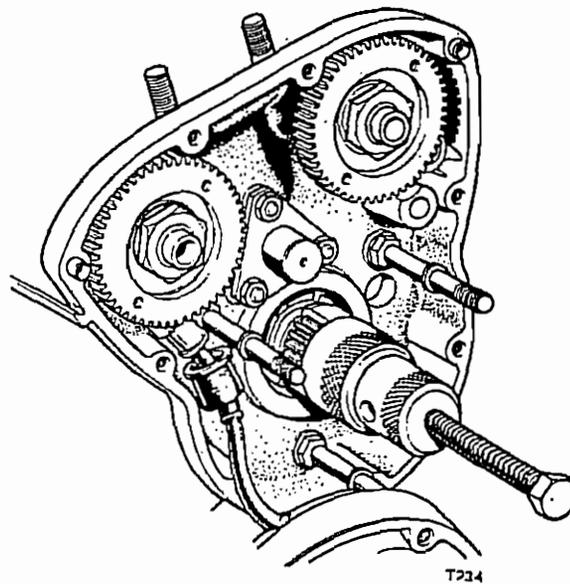
Fig. B32. Extracting the crankshaft pinion
