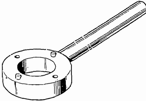
61-3694 Wheel bearing retainer peg spanner
