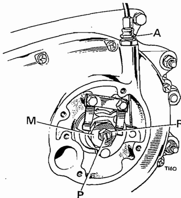
Fig. C2. Showing clutch adjustment
