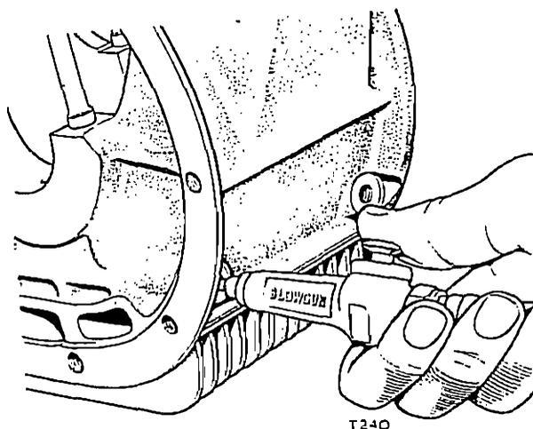
Fig. B36. Cleaning the crankcase oilways
