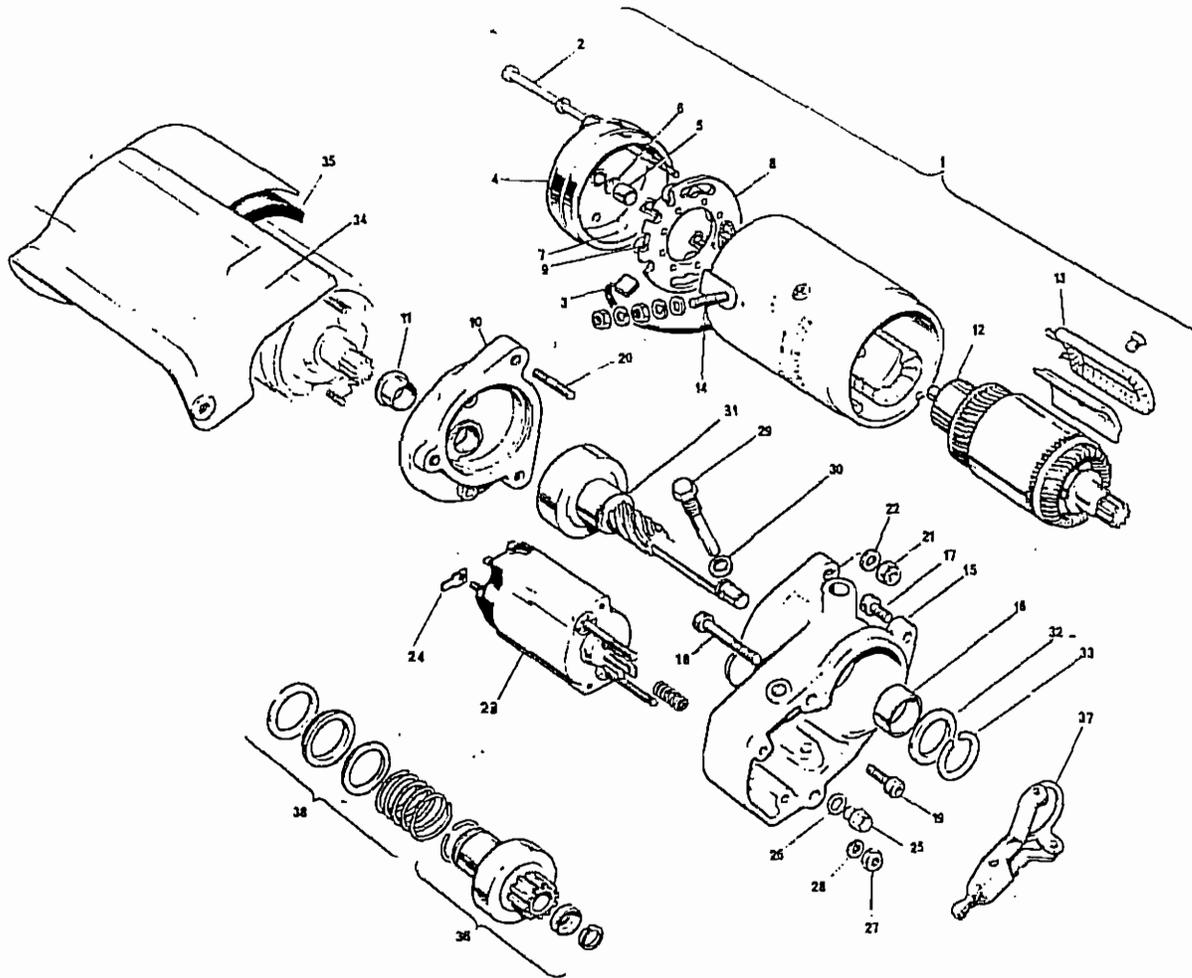
Fig. H27. Electric Starter Mechanism
