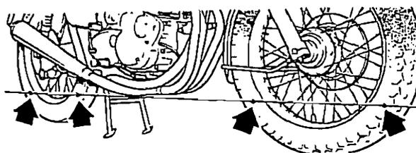
Fig. F11. Checking the wheel alignment
