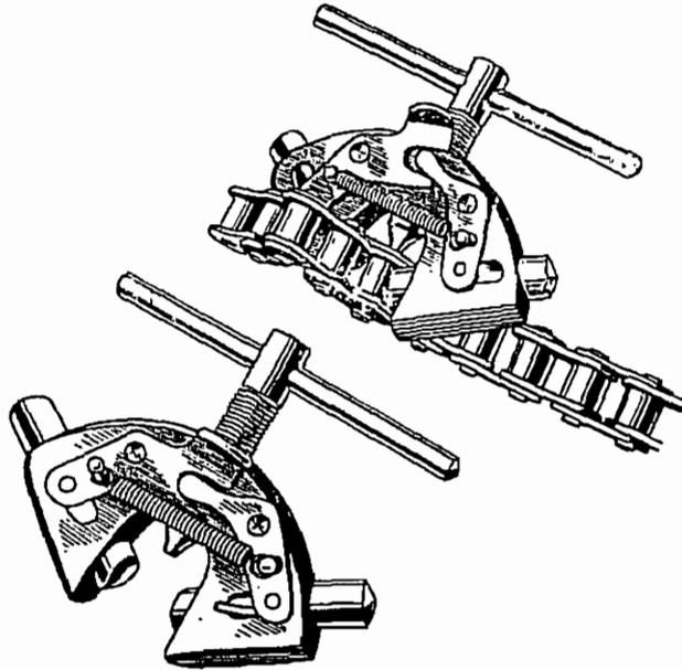
Fig. C12. Chain link rivet extractor,
