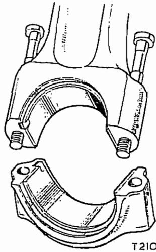
Fig. B38. Refitting a connecting rod
