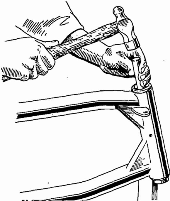
Fig. E10. Removing a swinging fork bush
