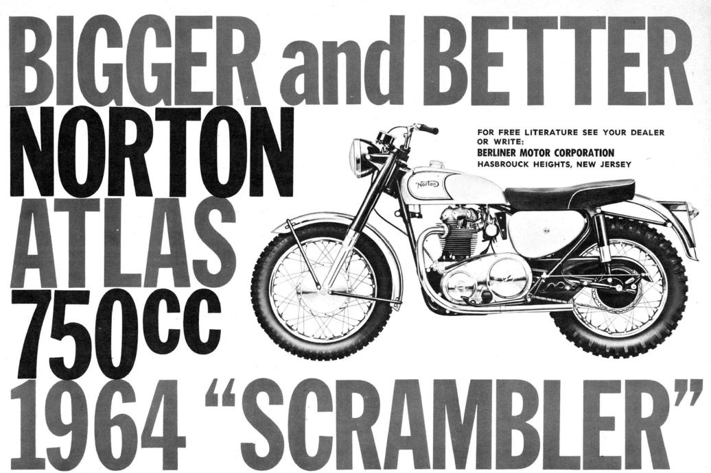
The 1964 Norton 750 "Scrambler" leaves nothing to be desired . . . Special rubber-mounted two gallon fuel tank . . . heavy duty spokes . . . Steel wheel rims chrome plated . . . Large full-hub brakes front and rear . . . Chrome plated front and rear fenders . . . special scrambles type handlebars re-inforced with cross member . . . Symetrically mounted speedometer and tachometer . . Folding kick-starter . . . Special "Road-holder" fork, heavy duty oil-damping springs housed in large diameter,
