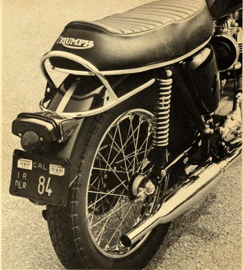
A large portion of the high speed handling characteristics come from the rear suspension system. Girling shocks dampen the rear portion of the chassis.
