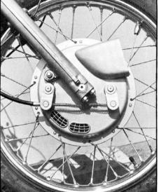
wheels add grace and beauty, while the new braking system brings the bike to a quick safe stop. The twin leading shoe on the front end is by far the best brake ever on a Triumph. The good handling characteristics can be attributed to the 56 inch wheel base and the comparatively light weight of 380 pounds. Power is quoted at 47 and seems fairly on the mark.
