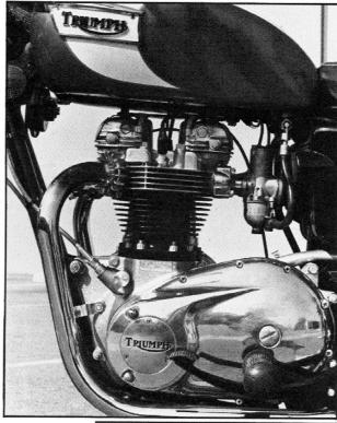
The only difference between the engines of the Tiger and the Bonneville is the single carb, which should make the Tiger reliable. One carb or not, the front end seemed very light under acceleration due to weight transfer. The new forks look like last year's racing options and do a fine job. Lucas seems to revel in having a poor reputation and, unfortunately, they support it again at Triumph's expense. Note the oil filler cap at the frame junction, just like a real racer.
