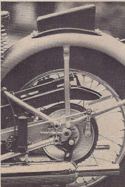
No hydraulic damping was used in the Thunderbird's unique rear suspension. The rigid frame models were, at this point, fading fast, as they were not as comfortable as the newer sprung hub model. Travel was here limited to 2½ inches.
