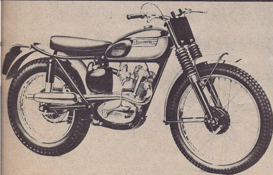
A pretty bike with trim lines, the 1962 TR20 was a 215 pound trials bike that featured a 200cc engine, four speed gear-box, and 8 inches of ground clearance.
