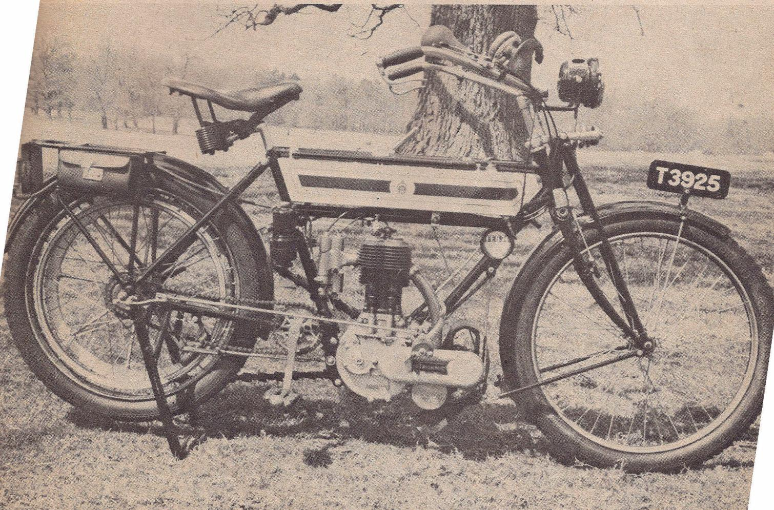
In 1911 Triumph produced this 500cc single speed single that had a clutch in the rear hub. The engine featured side valves and a manually operated oil pump.
