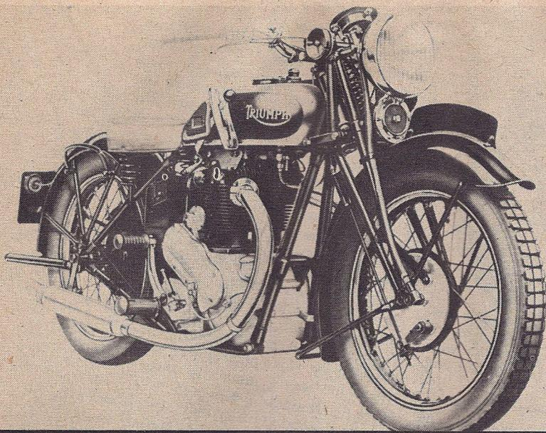
A dismal failure, the 1935 vertical twin had a hand shift in an era when the other British bikes all had a foot shift.
