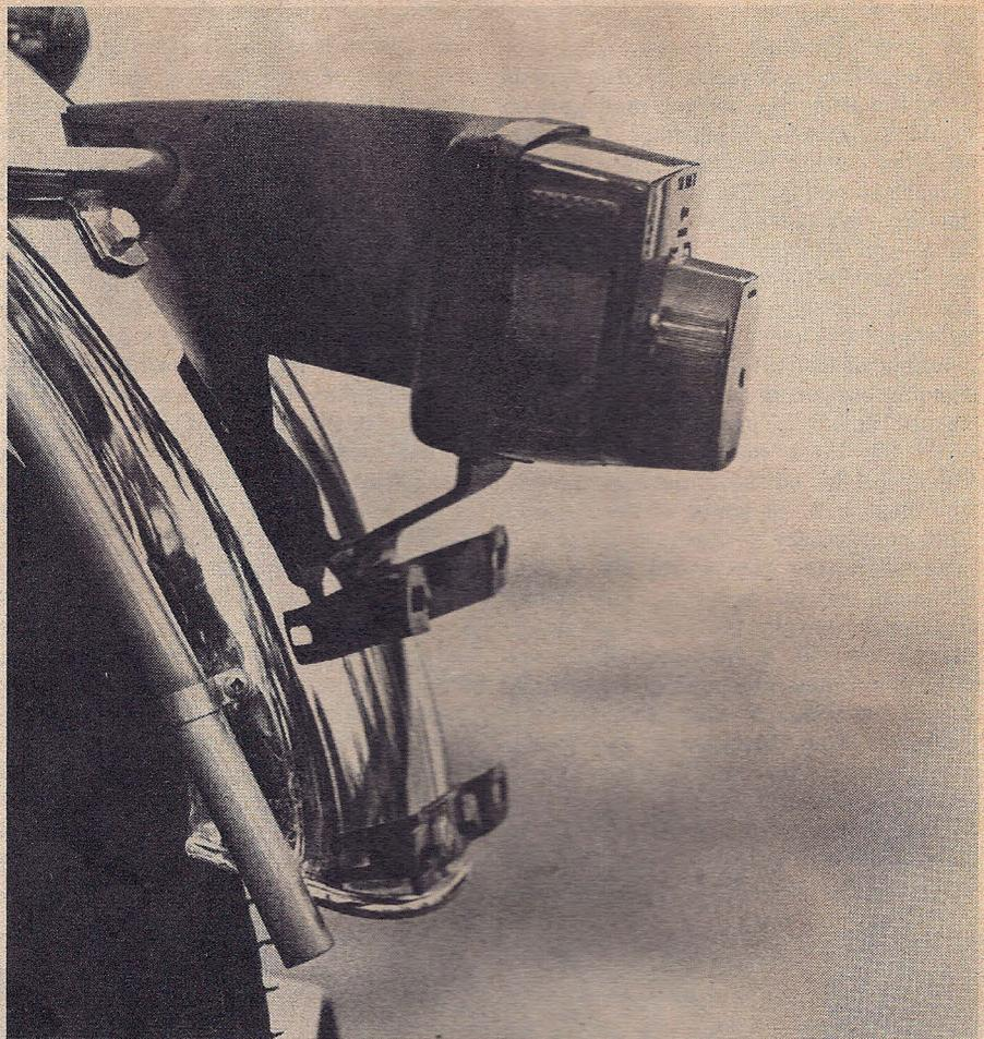
Note the crankcase breather hose vents below the rear fender eliminating oil mist residue.
