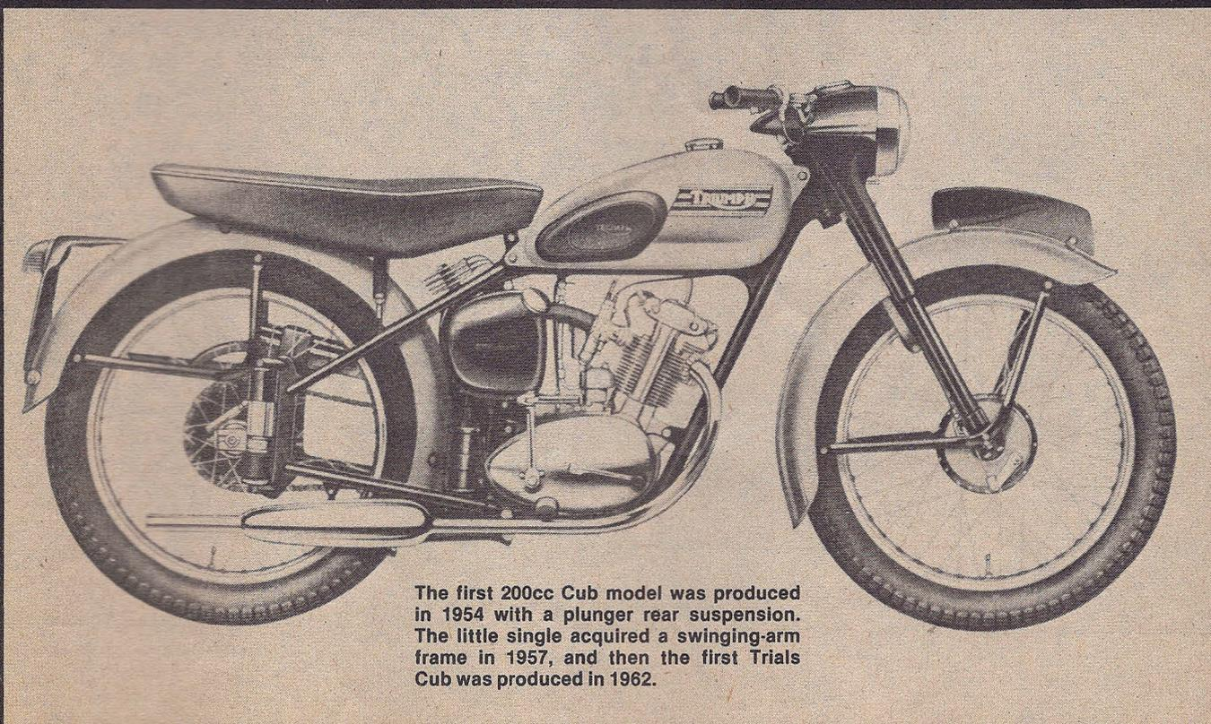
The first 200cc Cub model was produced in 1954 with a plunger rear suspension. The little single acquired a swinging-arm frame in 1957, and then the first Trials Cub was produced in 1962.
