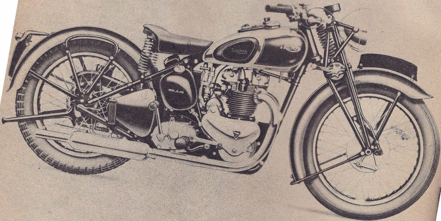
The model that revolutionized the industry—the 1938 Speed Twin. The 500cc twin had a compact engine and weighed only 365 pounds.
