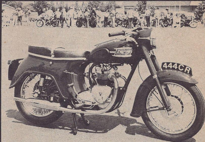
In the late 1950s Triumph produced the Speed Twin with large fenders and some enclosure of the central section. The idea was a failure.
