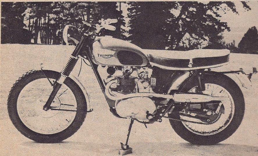
The 1966 Tiger 100 S was a 335 pound street-scrambler with the short stroke engine and an upswept exhaust system.
