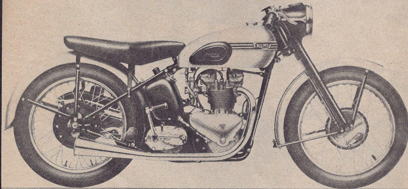
In 1951 Triumph produced a kit of parts to convert the Tiger 100 to a road racer. Many of these twins were raced with great success on America's dirt tracks.
